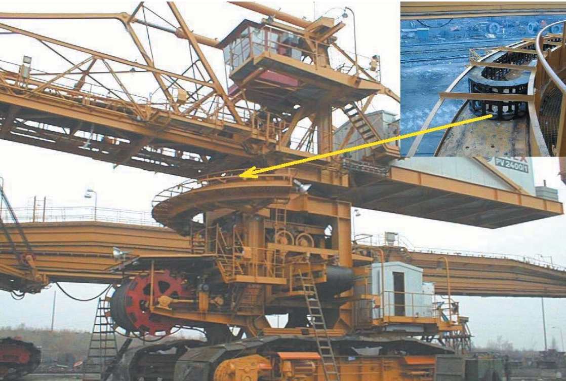
A rotary application on a bucket-wheel excavator uses an Energy Chain System®.
