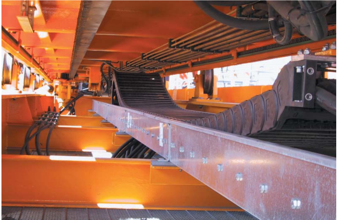
A pipe handling application protects its power supply with Energy Chain®.
