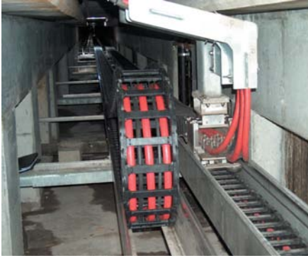
Floating towing arm, counteracts misalignment
