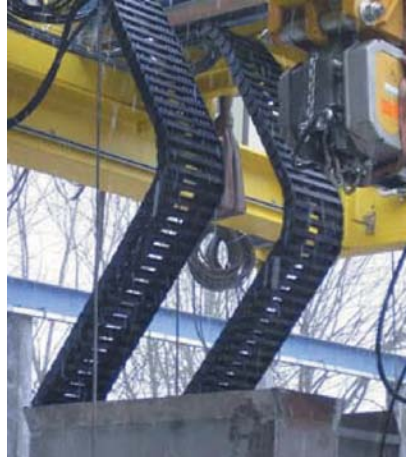
A challenging zig-zag application for the decommissioning of a nuclear power plant
