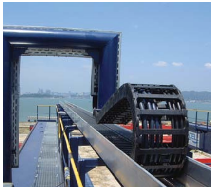
Crane builder with a travel of 63.9 ft and speed of 196 ft/min
