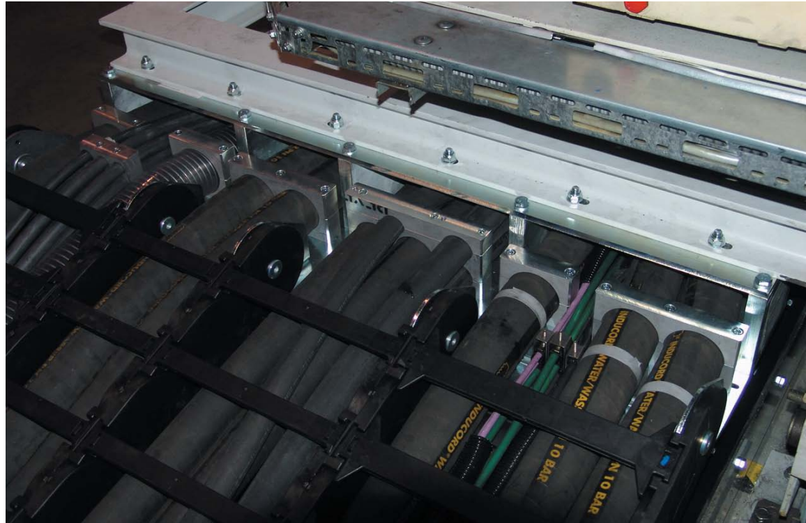
High additional loads are placed on the carrier due to high number of hoses and cables.
