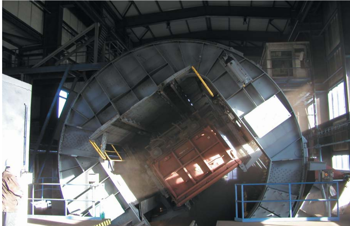
The bucket is turned 180° with the help of an igus® Energy Chain System®.
