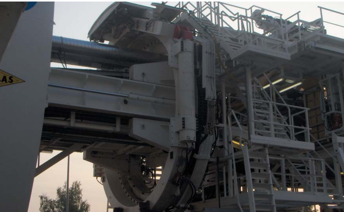
A tunnel drilling machine gets its power through an Energy Chain®.
