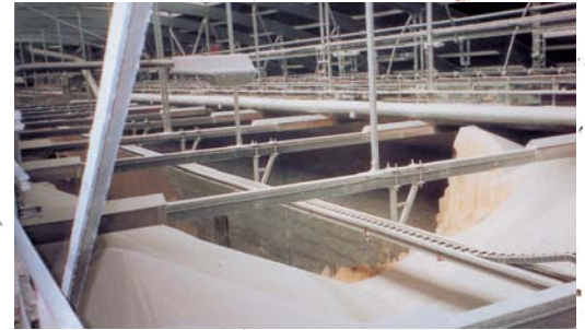
An Energy Chain®, in operation since 1998 at a fertilizer plant
