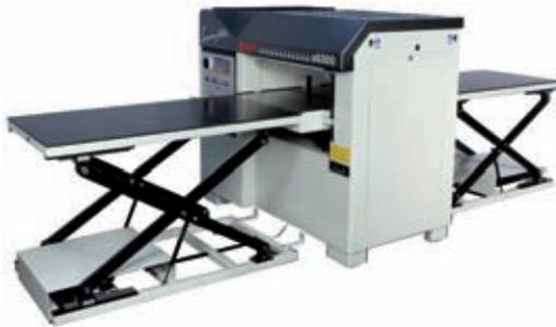
Also in this application, metal ball bearings were replaced by an igus® solution. Noise-free and precise DryLin® T-rail guides provide clearance for adjusting the height of the work tables. Large work pieces to be processed can be positioned on both sides of the machine. The tables are then adjusted to the height of the machine.
