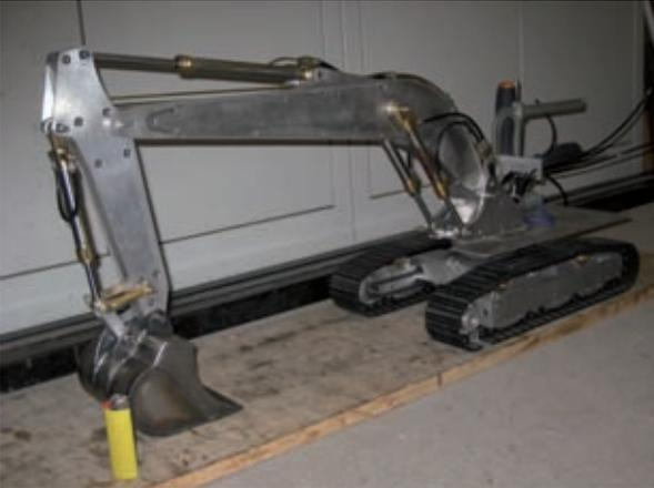
This fully functional hydraulic excavator was copied on a scale of 1:14.5. The model was based on the Liebherr type 954C. The model includes plain bearings made of iglidur® G, some of which are used to support the rollers in the caterpillar chassis. The igus® bearings increase the service life of the bolts and cylinder bearing points and are less expensive than comparable sintered bearings.
