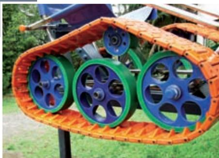
This special wheelchair allows people who can only walk with difficulty to go to the beach. For this purpose, it has been fitted with plastic chains instead of wheels. The axles are supported by iglidur® bushings. The ball bearings previously used did not even last a week against the aggressive sand and seawater conditions. In contrast, the iglidur® bushings are doing the job without any problems.
