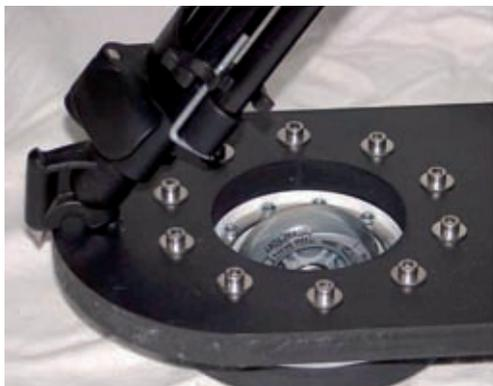
Another newly developed dolly for camera movement is the subject of this manus® contribution. It is suitable for all camera movements on smooth flooring. The dolly's rotation point is the point at which the three imaginary extensions of the wheel axes meet. The three casters in the bases have one iglidur® PRT rotary table bearing each. They can be adjusted in such a way that the dolly can be moved in any direction or be rotated around any one point.
