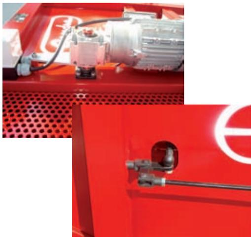
This machine cleans and sorts all types of grain. First the grain is separated from other material by an air current. Further sorting is done by various sifters. The components have to be as maintenance free and durable as possible. It is also desirable that the unit be lubrication-free, so that the grain is not contaminated. Therefore igubal® rod ends and iglidur® plain bearings are used, which meet all requirements.
