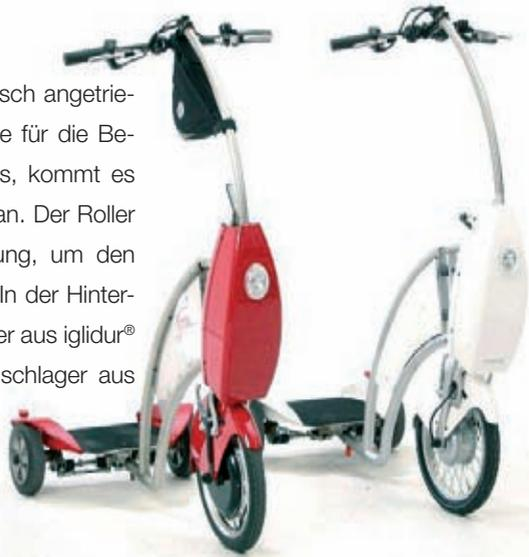
This three-wheeled scooter has an electric drive. Lightweight components are particularly important here to ensure as little energy as possible is required for movement. The scooter has additional rear-wheel steering to keep the turning circle extremely small. Two flange bearings made of iglidur® G were fitted in the rear-wheel steering, and flange bearings made of iglidur® M250 are also used.
