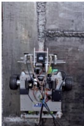
This small vehicle adheres firmly to surfaces with its magnetic wheels, to inspect welding joints. This enables it to reach especially difficult-to-access places. Environmental conditions include contact with water and ferromagnetic particles. This has to be considered in the wheel bearings. Therefore iglidur® plain bearings from igus® are used.
