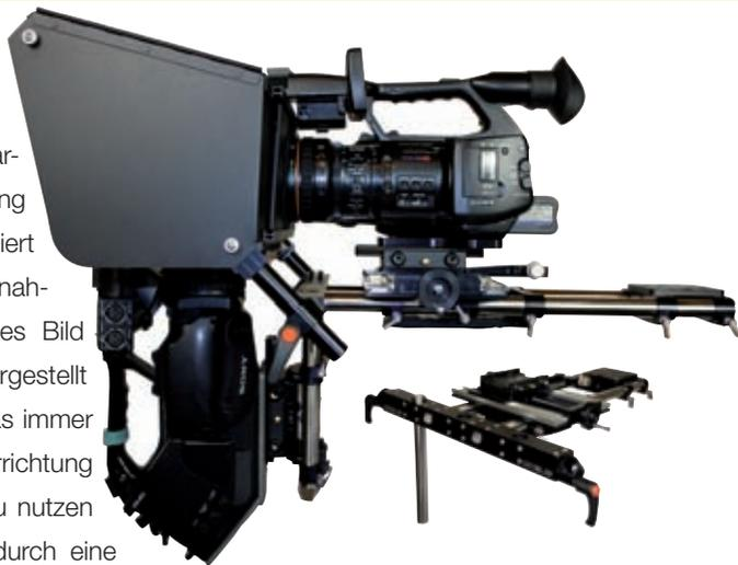
Instead of using expensive 3D cameras, two regular cameras can be mounted on this device so that together they can generate a three-dimensional image. The distance of the cameras must always be identical. A DryLin® N flat track was used to make the device itself easy to use and maintenance free.
