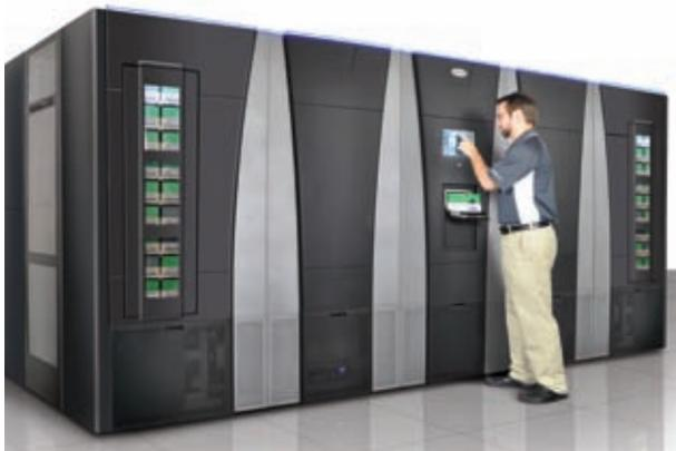
This machine manages data back-up tapes. The transport movements inside are guided by DryLin® N linear guides. These allow fast movement at low costs. Thanks to their especially small design height, even large-format tapes can be transported through the machine. Another convincing feature of the DryLin® N linear guide is its high reliability which means no maintenance work is required inside the machine.
