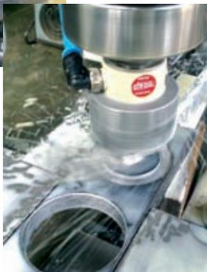
In the second application, an upright plastic ring is used to pick up and forward cooling emulsion in the machining process. This allows a smooth supply of cutting emulsion to the rotating cutting tool even at high speeds. The plastic is resistant to coolant and is thus not subject to any wear.
