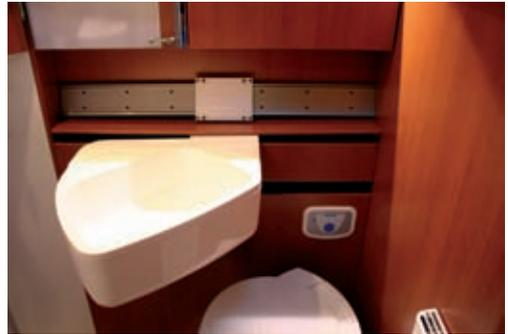
Every square centimetre counts when it comes to equipping mobile homes. Here, sanitary elements in the bathroom unit are installed with igus® products. The sink has been positioned so that it can be moved. A DryLin® double rail guides the movement. The toilet can be stored in the bathroom unit wall. An aluminium DryLin® precision shaft and the matching iglidur® plain bearings were used for maintenance-free pivoting of the toilet.
