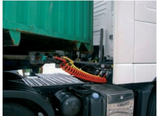
This application makes it possible to fit trailers of different lengths to prime movers. The cables used to connect the prime mover and the trailer have to be flexible to compensate the different trailer lengths. A combination of DryLin® W rails and DryLin® R plain bearings offers a space-saving solution here. This allows the driver to simply adapt the cable length without tools being necessary.
