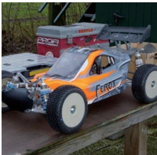
The suspension pins in this racing car were previously guided without bearings. This led to increased friction and excessive play in the chassis, which in turn affected performance. Now, the entire chassis is mounted with plain bearings from iglidur® J. They operate reliably in all environmental conditions. Since they show little wear, they are also a cost-effective solution for those who use this application as a hobby.
