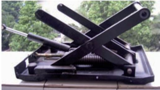
igus® plastic plain bearings are used here in the shock absorber of an excavator seat. Construction machines often encounter large loads and vibrations. The bearings that were previously used did not meet the requirement of stability and durability. But lubrication-free igus® bearings withstand the harsh environmental conditions of dust and dirt.
