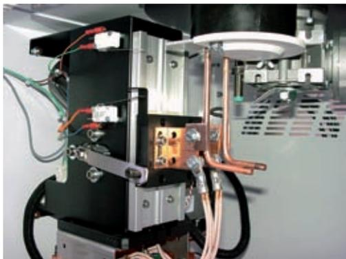
This newly developed induction centrifuge melts alloys for dental prostheses. For up-and-down movement in the device, the designers were looking for a linear guide that is economical, space-saving and maintenance free, and allows quiet motion of the slide-in tray with the inductors. A DryLin® N flat track from igus® is used here, and meets all the requirements
