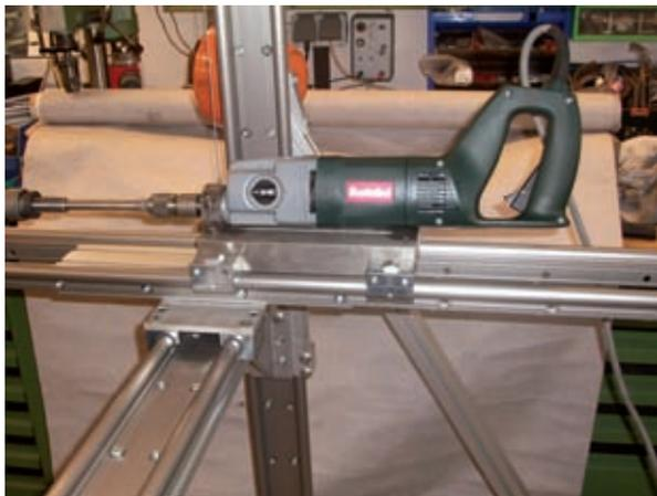
This frame construction allows the user to move the clamped tools, such as welding or milling equipment, along three axes, as desired. Thus, the physical effort is considerably reduced and handling of the tools becomes much simpler. This in turn increases safety. DryLin® W double-rail systems were built in on all three axes.
