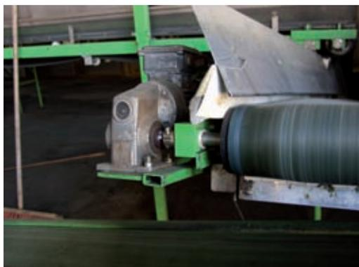
This machine is used for preparing and drying kitchen herbs. Up to now, soiled and non-functioning belt scrapers, faulty ball bearings and worn shaft ends on belt cylinders caused machine downtime. With special parts made of iglidur® for the belt scrapers and regular iglidur® plain bearings as a replacement for ball bearings, the downtimes have been significantly reduced.
