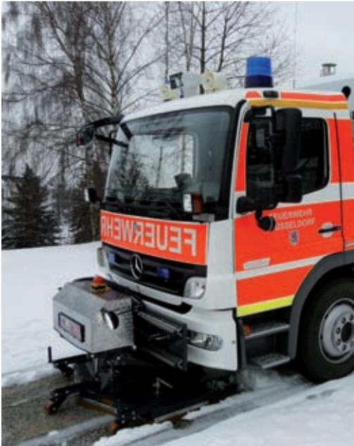
This machine is used for the elimination of high levels of soiling. It is mounted to a vehicle and sprays a mixture of water and cleaning agent onto the road at high pressure, and then draws it off again using a vacuum. A low-cost linear plain bearing with a long service life was required, which can compensate alignment faults and is as light as possible. The solution: an igus® DryLin® R-aluminium shaft.
