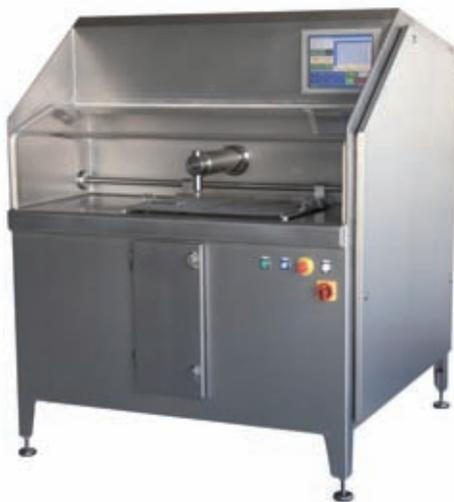
Maximum care must be taken with hygiene wherever foodstuffs are handled. This machine cuts foods of all kinds into all sorts of pieces and patterns. This is even possible with the food still frozen. The combination of igus® DryLin® linear plain bearings and stainless steel shafts makes cleaning the machine easy. Since no lubricants are involved, there is no danger of product contamination whatsoever.
