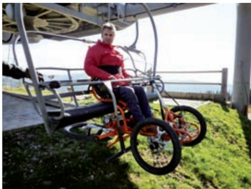
This manus® contribution also offers an exceptional off-road wheelchair, the Quadrix. It was designed so that disabled people can use a ski lift or chair lift while sitting on it. This requires simple, but robust and low-maintenance components for the joints. So all front axles are fitted with igus® plain bearings.
