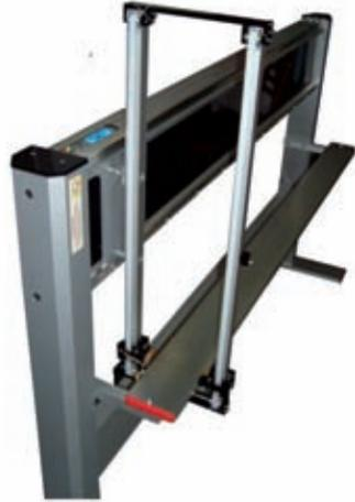
This computer-controlled foam cutter manufactures decorative objects. The foam blocks are cut with a hot wire. The cutting wire is moved along the vertical axis by two DryLin® ZLW toothed belt shafts. This solution replaces the previously used ball bearings, which are more difficult to make and were particularly susceptible to dirt.
