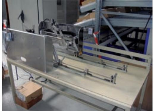
This machine is used for loading and unloading of boxes at an automated warehouse. The gripping arms are controlled linearly by motors, and extend a telescopic rail along the load to be moved, so that it is loaded onto or removed from the carriage that traverses the high-rack warehouse. The grippers are equipped with iglidur® plain bearings. These work reliably even in the somewhat dusty environment of the warehouse.
