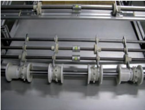
This equipment is used in the food industry. The baked goods are separated on these chains. A lubricant-free mechanism is essential because of the flour dust and the direct contact with food-stuffs. Therefore iglidur® J flange bearings and DryLin® trapezoidal leadscrew nuts are used. The linear movements are guided by DryLin® N rails and slides.
