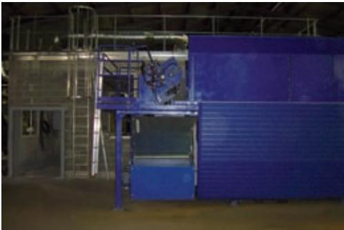
This machine is used for the improved recycling of domestic waste. It opens refuse bags and roughly pre-sorts the contents. The easier material flow is designed to make subsequent recycling easier. An igubal® flange bearing guides the components used to open the refuse bags. Each machine contains 69 igubal® flange bearings, which were chosen on account of their corrosion resistance, lubricant freedom and space-saving design.
