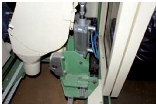
The head sections for large wooden wine barrels are sanded in this machine. DryLin® T-rail guides are used to position the grinding heads. DryLin® W profile guides control the movement of the brushes and the sliding doors. Further pivoting movements are carried out with iglidur® G flange bearings. All igus® products used are maintenance-free, giving the machine a long service-life.
