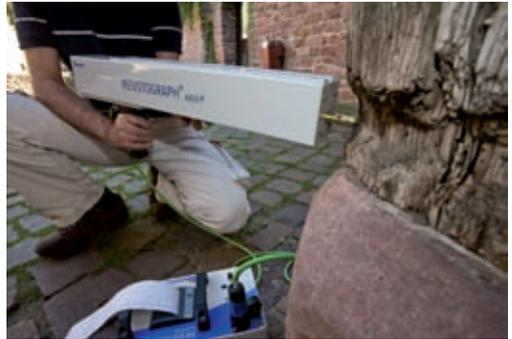
This device measures the drilling resistance of a needle penetrating wood at high rotational speed. It allows the inner condition of trees and timber to be determined almost without destruction. The devices are exposed to different temperatures and drilling dust during the process. Conventional rail guides were too heavy and relatively high-maintenance. The change to a lubricant-free igus® rail guide allowed the device to be made smaller and less expensive.
