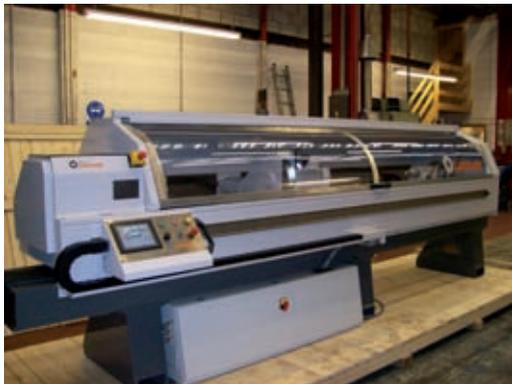
With this drum sanding machine, the console should be able to be positioned in any position along the front. For this purpose, all the operating elements must be attached directly to the machine to achieve a real stand-alone solution. The DryLin® W linear guide used as a double rail more than four metres long, making adjustment of the console easy. An E-Chain® is a further igus® product used to protect the cables.
