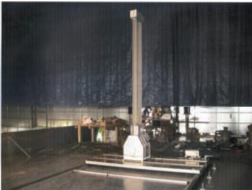
Here in a shielded hall, trains are tested for their electromagnetic compatibility. This requires the testing equipment to move along the total length of 42 metres. Because of the uneven ground, a tolerance-compensating DryLin® W rail system is used. The system is robust, for it is mounted on the ground, and it can even be entered.
