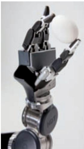
This robot arm is so strong that it can use a drill. Yet its movements are so sensitive that it can even handle raw eggs. Since the arm itself has to be as resilient as possible, its own weight must be reduced. High reliability of the components is also important. The developers decided to use plain bearings, flange bearings and thrust washers from iglidur® G in the joints.
