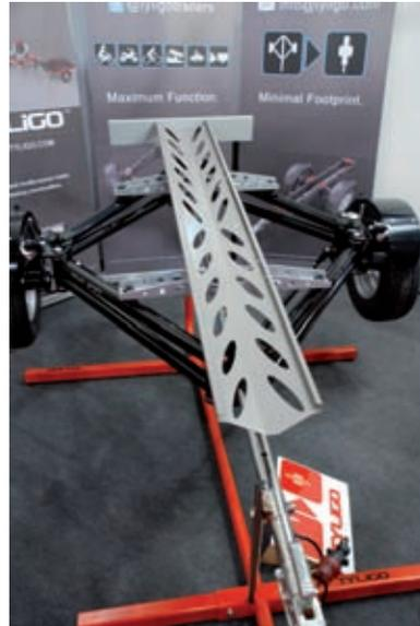
This folding trailer “Tyligo” is extremely flexible and can be used to transport all kinds of things. There are versions for bike or motorbike transport available, with loading areas for general transport and even a version for jetskis. The special thing about it: the trailer can be folded up neatly when it is not used, saving space. One igus® plain bearing and 18 thrust washers made of iglidur® G are used in the folding mechanism.
