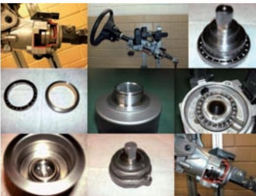
In this application, plain bearings made of iglidur® Z replace a ball bearing and a needle bearing in a superimposed transmission. The transmission permits steering angles to be added by the rotary movement of an electric motor in the same or opposite direction in addition to the steering wheel angle chosen by the driver. One of the benefits of using lubricant-free plastic plain bearings is that it ensures the transmission can be fitted more quickly.
