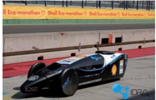
This racing car is powered by hydrogen. For the most efficient fuel consumption, weight was reduced wherever possible, while minimising the rolling resistance. The steering unit, inclusive of the steering rod, is made of carbon fibres and is mounted with igubal® flange bearings and igubal® rod end bearings. These allow a weight reduction of about 30 per cent compared to other solutions.
