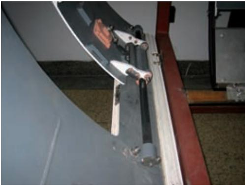
At a speed of more than 350 kilometres per hour, these trains will be racing through China as of 2012, connecting Beijing and Shanghai. The movement of the train doors will be guided by DryLin® R linear plain bearings. The designers opted for the igus® bearings, because they wanted to build a lubrication-free and thus low-maintenance mechanism, which is also quiet and operates reliably in all weather conditions.
