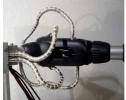
In this case, the design for a 5-axle jointed arm was submitted to the manus® competition. The jointed arm was constructed with two robolink joints from igus®. With robolink, different movement mechanisms are integrated in one component, the actuators and control modules are decoupled from the tools. The fifth degree of freedom is provided by a servo motor. An electromagnetic gripper is used as a "hand" here.
