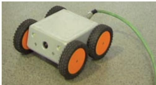
This robot checks ventilation shafts before and after cleaning. By using iglidur® W300 plain bearings, reliability can be increased. The previously used ball bearings had to be oiled regularly, which is not the case with iglidur® bearings. Due to their small size, the robot could be smaller, so that even smaller air ducts can be expected. Using a DryLin® N flat track, a disinfectant injector can also be mounted on the robot.
