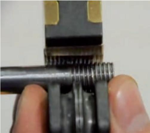
With this hand tool for the rolling and repairing of threads, the bearing support of the profiled roller is particularly important. The maximum feed forces that can occur can reach 1.2 tonnes. iglidur® Z plain bearings are used for this application, which, the design engineer reports, are the only bearings that fulfil the demanding requirements and have passed the endurance tests.
