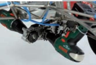
The driver lies on this vehicle with his arms stretched out and head facing forward. The vehicle accelerates to over 30 km/h and is steered by the driver shifting his weight. This necessitated the development of a completely new joint which is at the heart of the vehicle. The joint has to bear the load of the driver's entire weight. The joint is made up of several axes and braces. iglidur® JVFM plain bearings were selected for smooth and wear-free movement.
