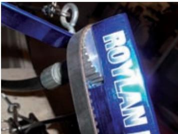
In this pedal boat, the moving parts of the drive mechanism have to have lubricant-free bearings because the screw is under water. Lubricants would be washed away permanently. This is where igus® plastic plain bearings are required. They guarantee the lubricant-free force transmission from the pedals via the toothed belt to the screw – which means no maintenance is required.
