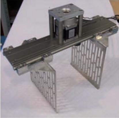
This gripper picks up freshly baked goods from a conveyer belt and packs them in baskets. The gripping movement is achieved using DryLin® W rails and DryLin® W slides. The slides are connected using igubal® double pivoting joints to ensure even movements of the two gripper arms. As always in the food industry, absolute lubricant freedom and cleanness have top priority for this application.
