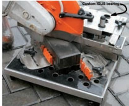
Here, a cutting machine for paving stones was submitted to the manus® competition. The application required a bearing that can be fitted or replaced quickly and can resist the dusty environmental conditions. A slotted oval plain bearing as a special part made of high-performance iglidur® met the requirements. It is used in the clamping fixture for the paving stones.
