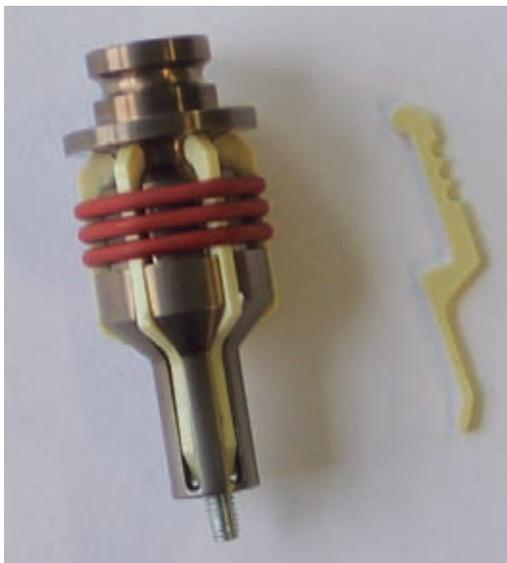
In this case, special properties of the iglidur® materials were used for a special part: for the gripper bracket for screws in automatic screwing devices – previously a job done by steel cheeks. However, these caused abrasion and channels on the screws to be processed. Geometrically identical cheeks made of iglidur® plastic prevent damage and chip formation.
