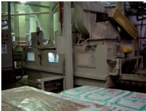
In this entry to the manus® competition, sacks containing asbestos are cut open automatically. Since asbestos is extremely damaging to the health, the procedure has to be carried out in a protective cabin. This means moving parts are difficult to access for maintenance purposes. For this reason, DryLin® linear guides and igubal® KSTM pedestal bearings are used; these need no maintenance and are not affected by the aggressive asbestos either.
