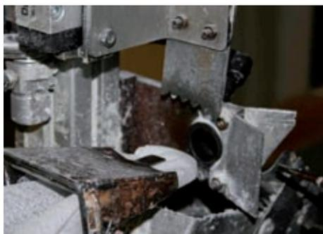
This manus® contribution makes an unusual use of iglidur® flange bearings: for winding cotton wool. The end products include, for example, balls for crafts, balls for throwing and dispersion carriers. The use of iglidur® bearings quadrupled the service life of the machine, and made it possible to save almost 300 mechanic-hours plus ca. 8 tonnes of cotton wool. The material savings are equivalent to about 40 cubic metres of wood.
