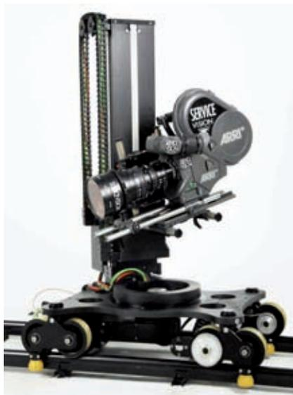
This camera dolly is particularly quiet and easy to adjust. It allows a wide range of different movements. Up and down movements of the camera are controlled by four DryLin® T-linear guides. This solution permits fast relative movements. In addition, the aluminium design of the DryLin® T-trails significantly reduces the weight of the dolly.
