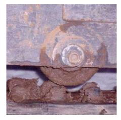
damage. iglide<sup>®</sup> G300 plastic bushings replaced expensive, grooved ball bearings and substantially increased service life due to their greatly reduced susceptibility to dirt and humidity. This application has been running problem-free and without maintenance for four years.
