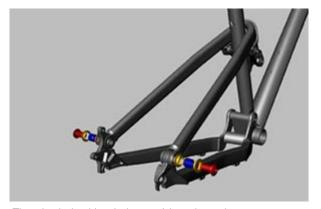
The plastic bushing is inserted into the swing arm and enclosed in a metal sleeve, which forms the end stop for tightening the screws.
