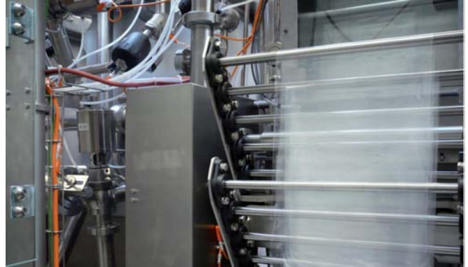
xiros® used in film guide rollers
