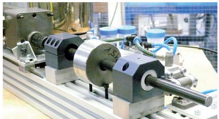
xiros® wear testing in igus® laboratory
