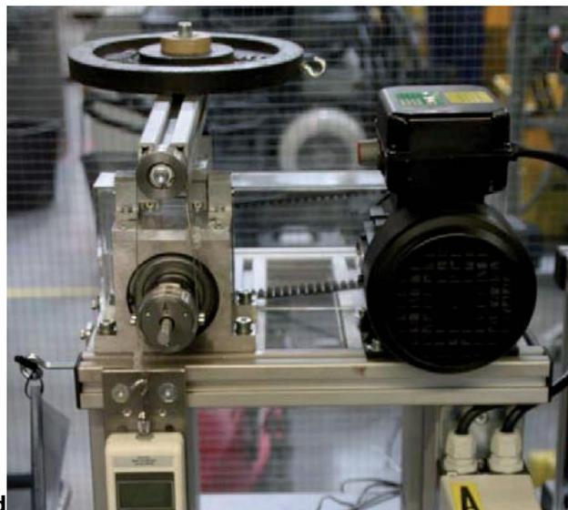
Diagram 1.2: Coefficient of friction test stand
