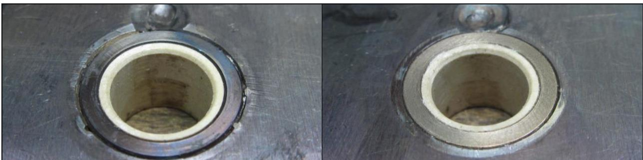
No measurable diameter reduction could be found on the plastic shaft. The smooth running tracks can be seen in diagram 3.
